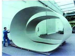
advantages. Separate pieces can be elastically deformed and then transported into tight spaces. At the point of installation, the parts can then be brought into their final shape and welded together.
